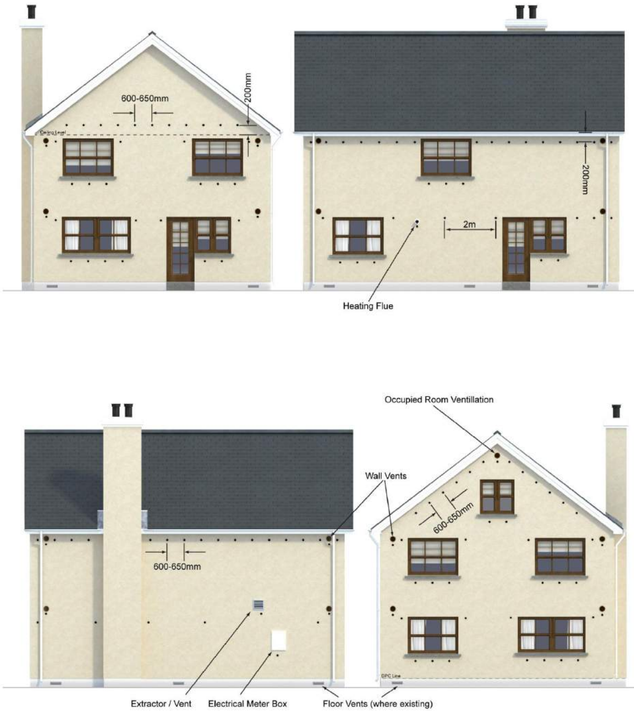
Figure 1: Typical KOREFILL Hole Drilling Pattern in a Detached Dwelling - New and existing buildings without existing partial fill insulation in cavity.
