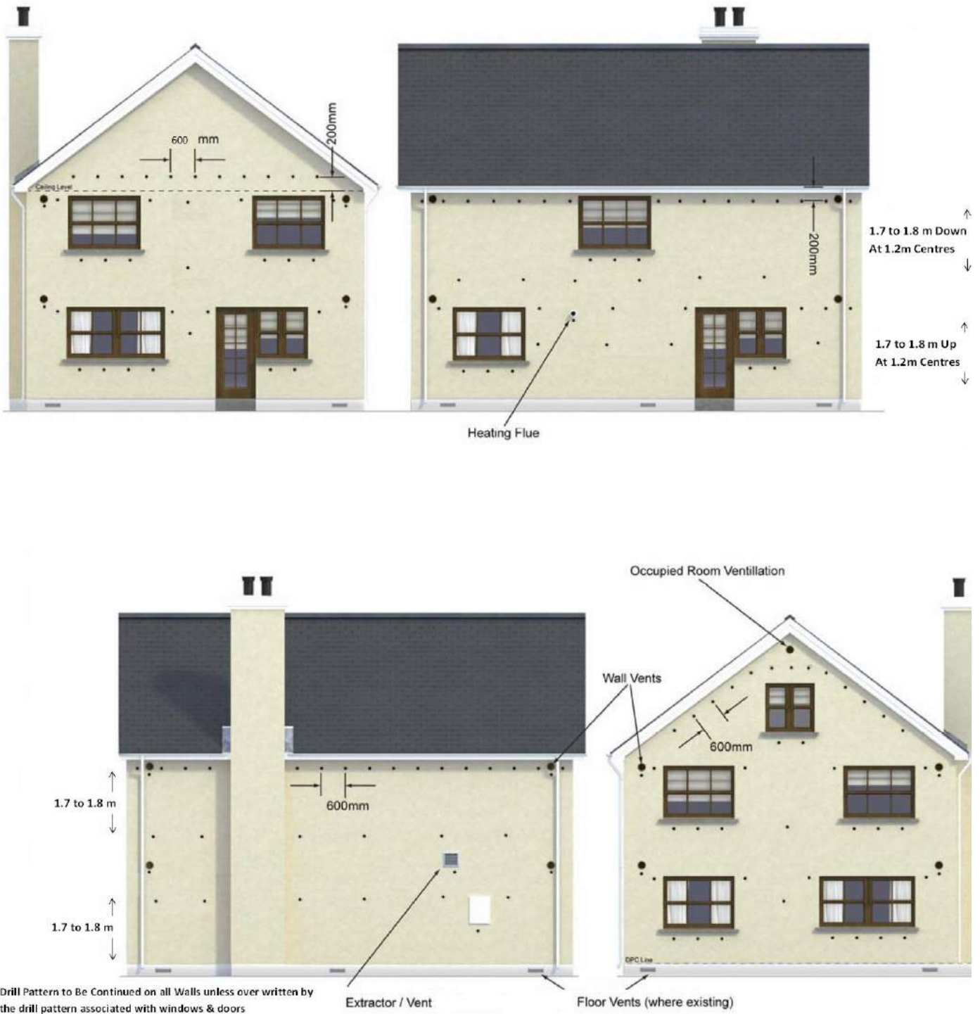
Figure 2: Typical KOREFILL Hole Drilling Pattern in a Detached Dwelling for Residual Fill Application. - New and existing buildings with existing partial fill insulation in cavity.
